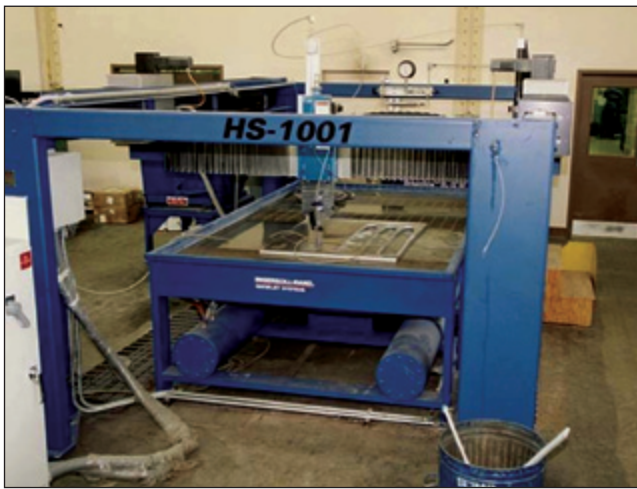
Figure 6. A waterknife designed to be 30 dBA quieter than an older version.
