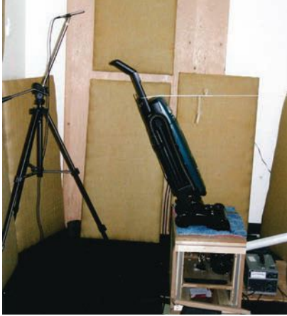
Figure 1: Use of a specialized test rig to impart representative loading on vacuum cleaner motor. Source: Acentech
