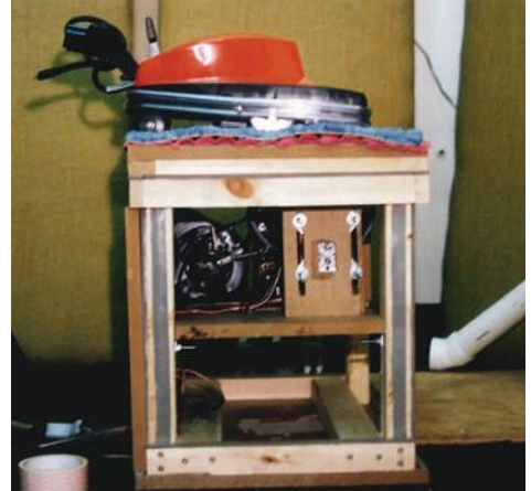
Figure 1: Use of a specialized test rig to impart representative loading on vacuum cleaner motor. Source: Acentech
