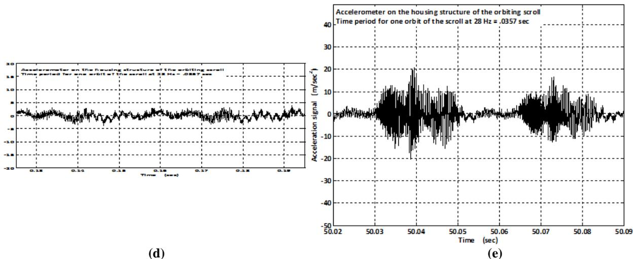
**Figure 2 (cont'd):** Housing acceleration signal, short time slices: d) just before "chirping" noise became noticeable; e) just before the sudden jump in amplitude
