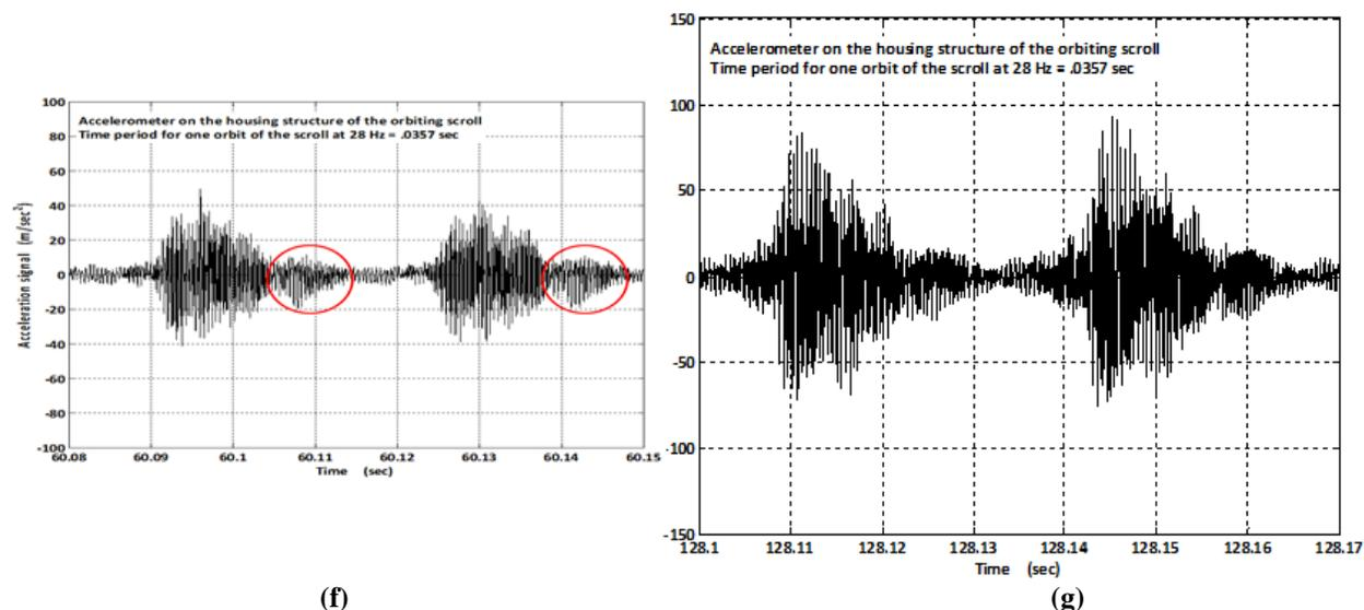
**Figure 2 (cont'd):** Housing acceleration signal, short time slices: (f) after the sudden jump in amplitude - red circles indicate a possible second pulse; (g) near the end of the plot in Fig. 2a
