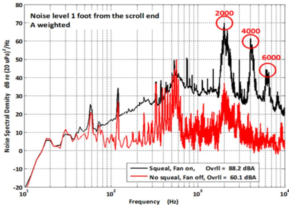
**Figure 2c:** Audible spectrum with and without "chirping" noise
