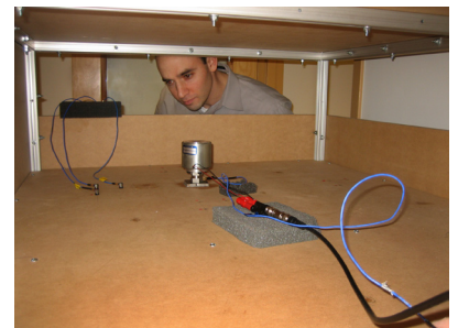
Scale model of a building with vibration source and measurement sensing equipment.
