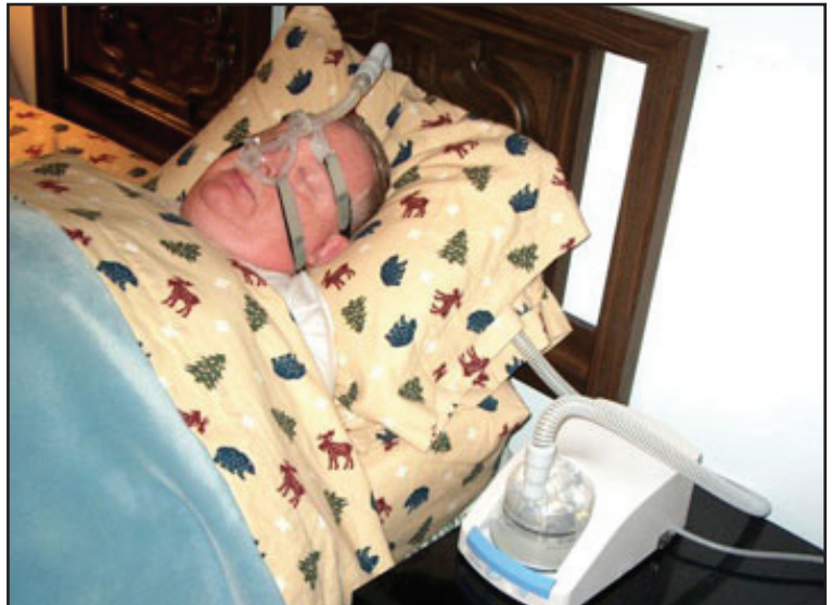
This photo shows how a CPAP system fits on the user, as well as the proximity of the base unit to the user, underscoring the need for quiet system operation. Source: American Sleep Apnea Assn.
